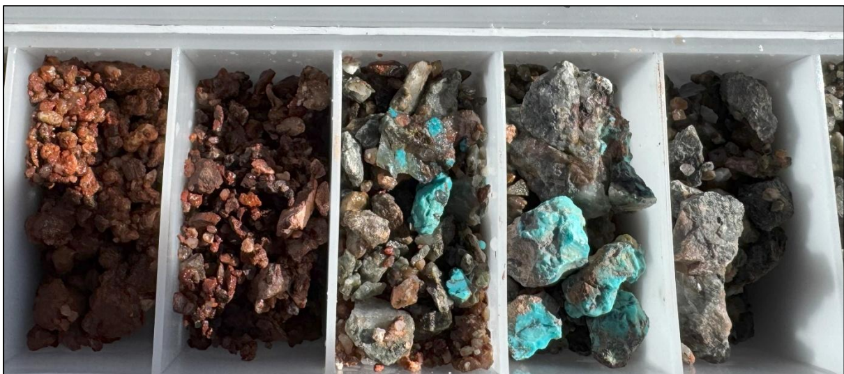
Figure 4: Copper carbonate mineralisation within oxidised structure in PRC010 (252 ft to 260 ft)
