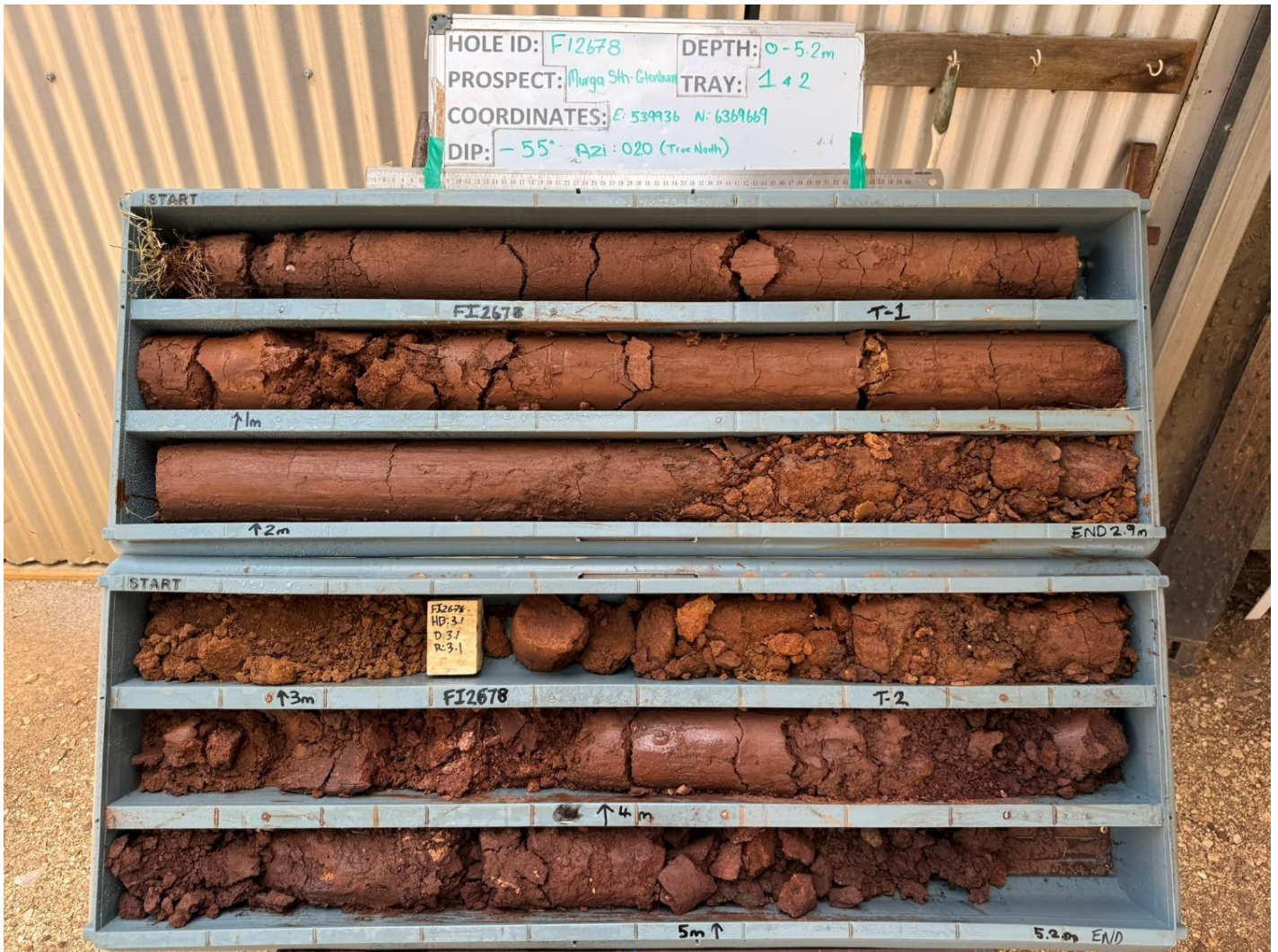
Figure 3: Photo of FI2678 PQ core – 0 to 5.2 metres (clay / laterite)
