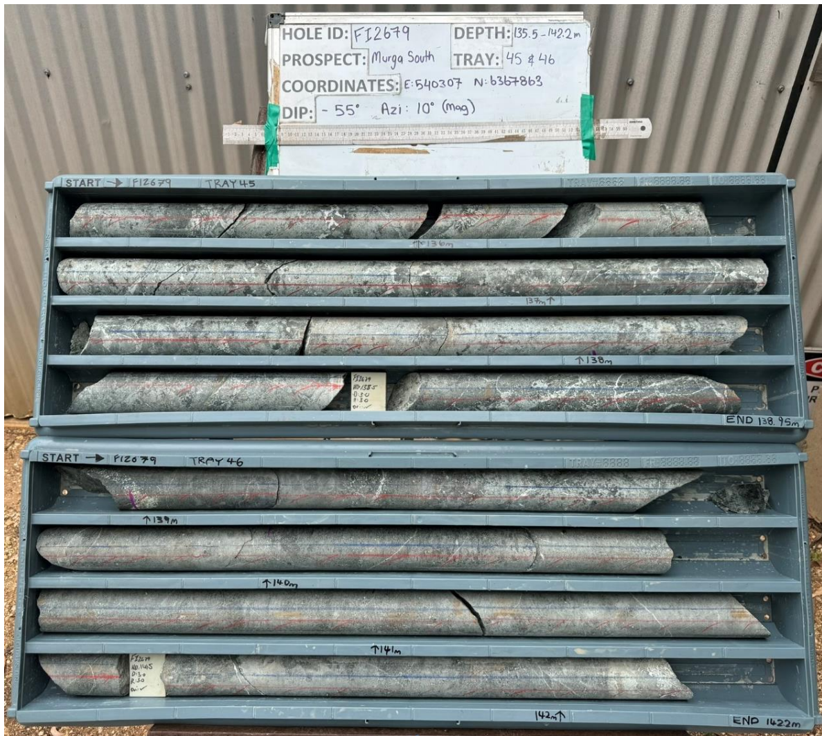
Figure 6: Photo of FI2679 HQ core – 135.9 to 142.2 metres (serpentinised pyroxenite)
